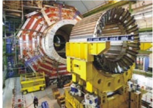
Core magnet of the Compact Muon Solenoid experiment at the European Organisation for Nuclear Research. Photo: internet
